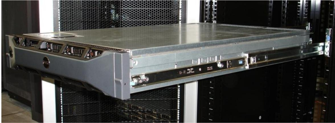
**Figure 12. R815 Mounted in the B2 Sliding Rails**
