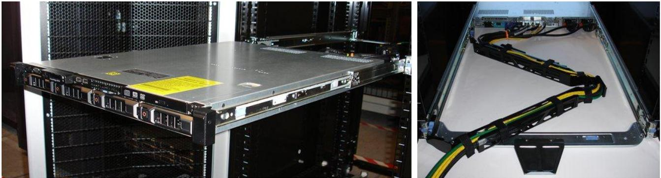
Figure 28. R410 Mounted in the A3 Sliding Rails with the CMA
