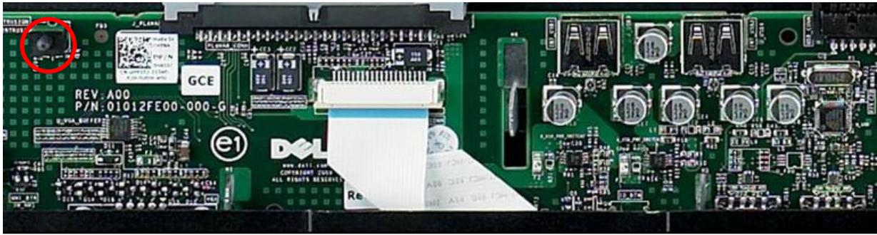
Figure 14. Chassis Intrusion Switch
