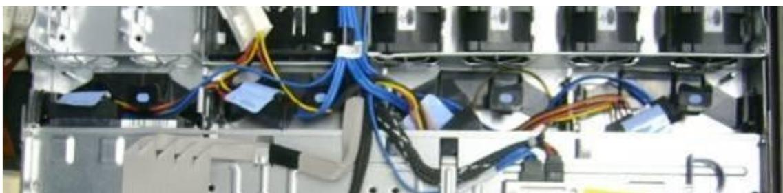
Figure 22. Top-View for Cabled HDD Connection
