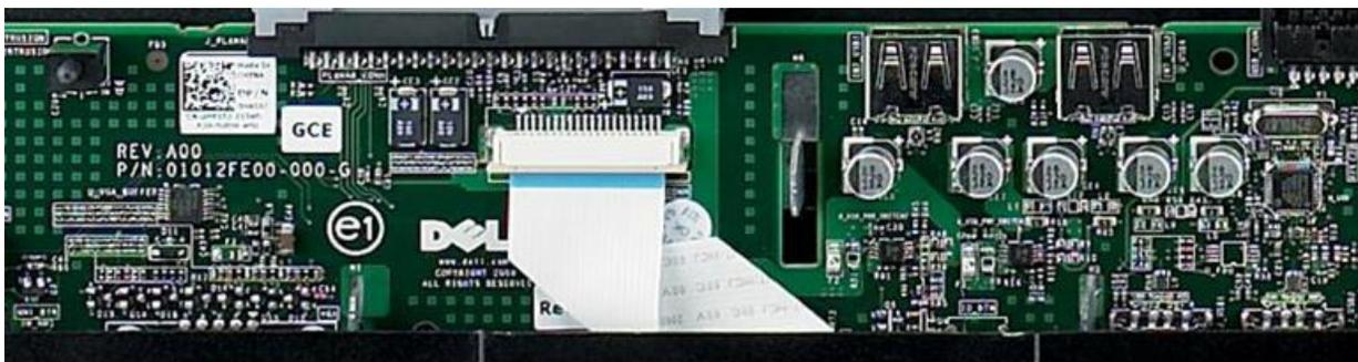
Figure 13. Front Controller Board with Diagnostic LED
