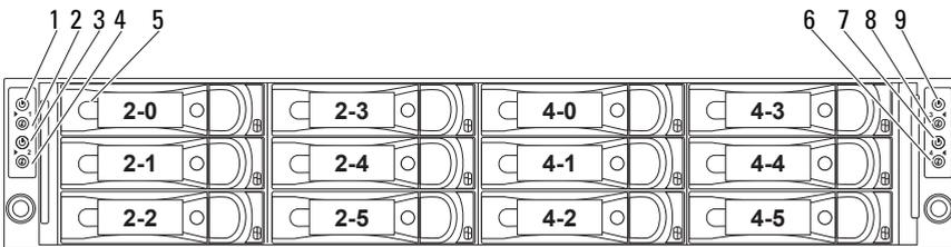
**Figure 1-4. Front Panel—2.5" Hard Drives With Four System Boards**
