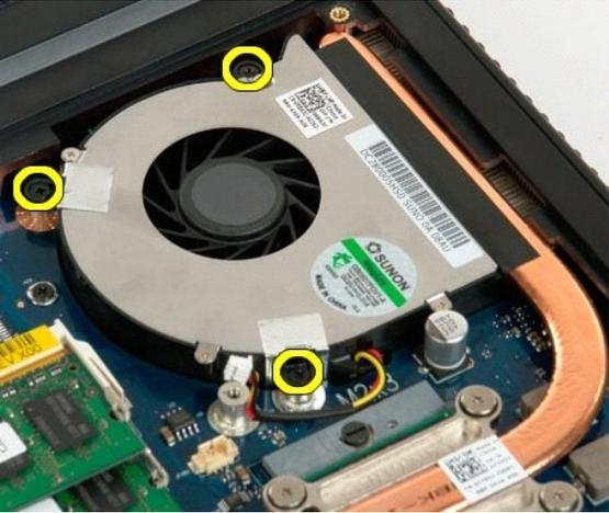
6. Lift up on the fan and remove it from the computer.
