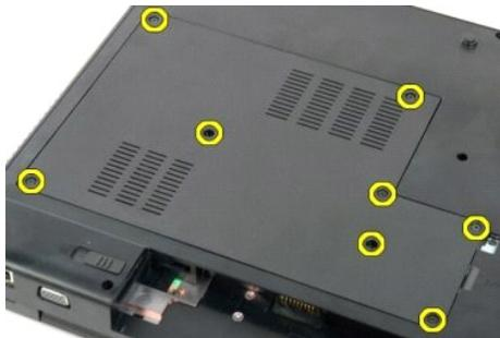
4. Lift the edge of the access panel that is closest to the center of the computer.
