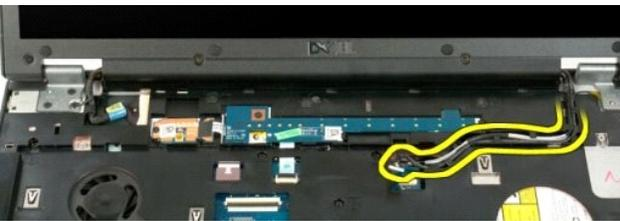
9. Disconnect the display data cable from the system board.
