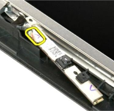
7. Remove the camera from the display assembly.
