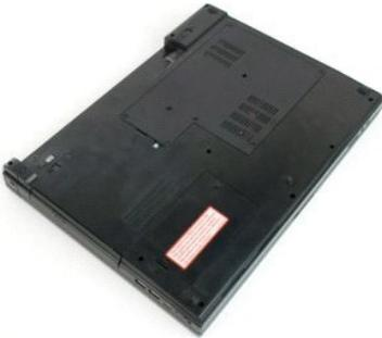
3. Remove the screw that secures the optical drive in the computer chassis.
