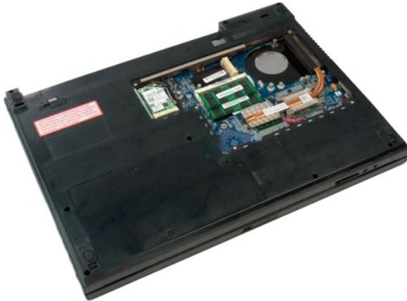
5. Loosen the four captive screws that secure the heat sink to the system board.
