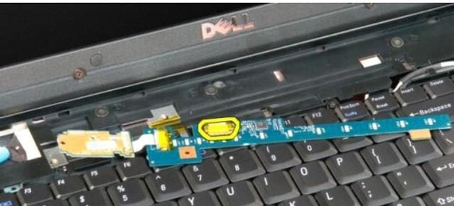
10. Remove the two button pads from the computer.
