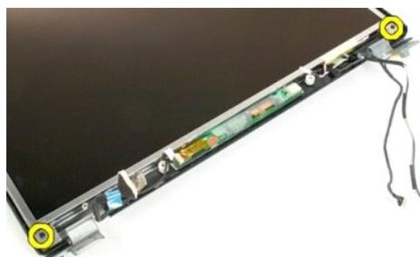
5. Remove the LCD display panel from the display assembly.
