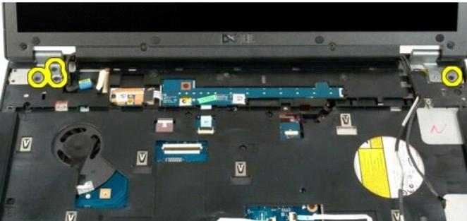
11. Lift the display assembly straight up and remove the display assembly from the computer.
