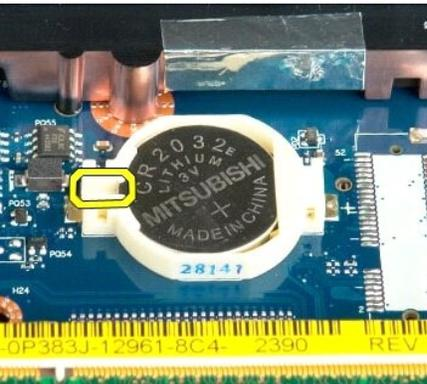
5. Remove the coin-cell battery.
