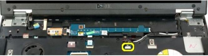
8. Remove the data and antenna cables from the palm rest.
