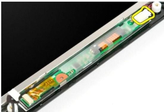
5. Remove the inverter from the display assembly.
