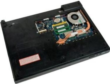
4. Disconnect the fan cable from the system board.
