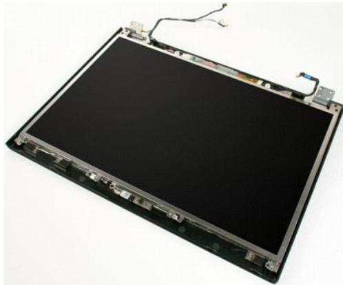
4. Remove the screw that secures the camera to the display assembly.
