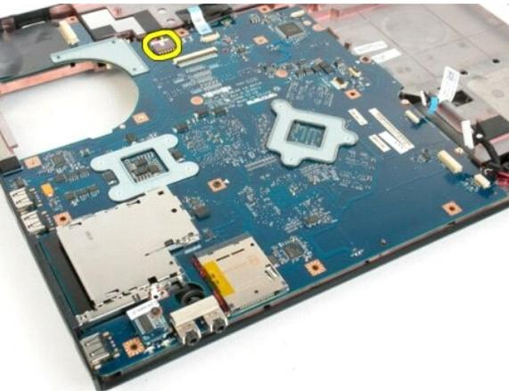
15. Remove the three screws that secure the system board to the computer chassis.
