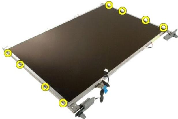
6. Slide the hinges away from the display panel assembly.
