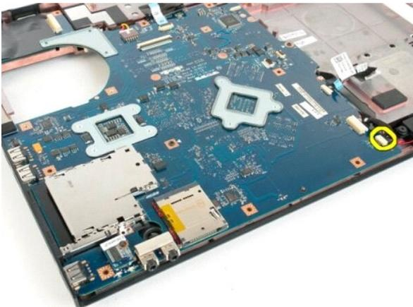
12. Disconnect the USB/IEEE 1394 data cable from the system board.
