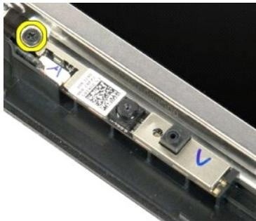
5. Lift the camera from the retention bracket.
