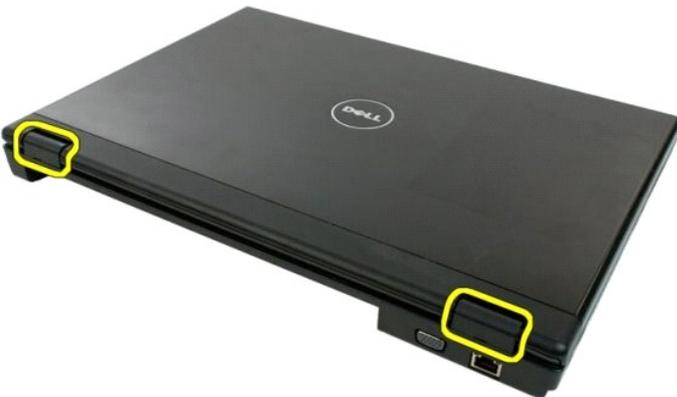
4. Starting on the right side, separate the hinge cover from the base of the computer.
