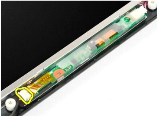
4. Disconnect the power cable from the display inverter.
