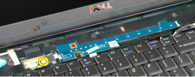
6. Remove the screw that secures the multimedia button pad to the computer.
