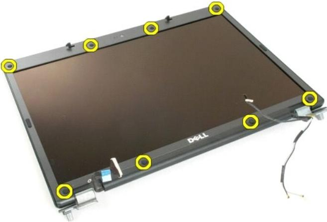
4. Remove the eight screws that secure the bezel to the display assembly.
