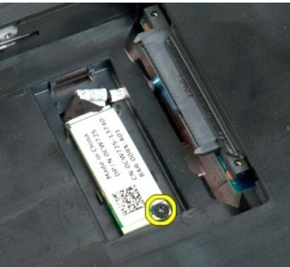
5. Lift the edge of the Bluetooth module closest to the front of the computer.
