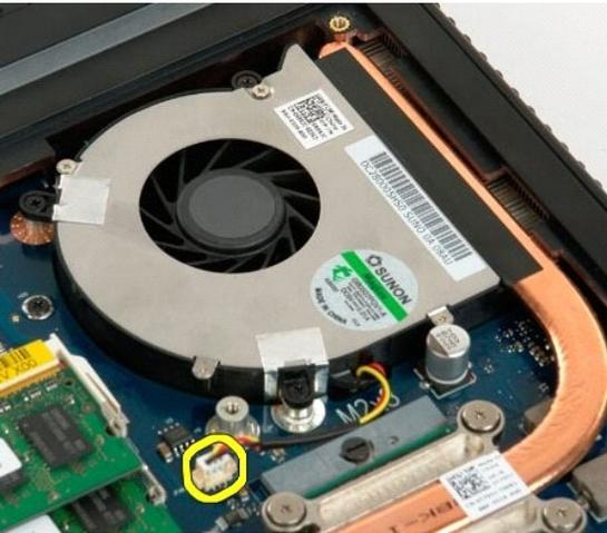
5. Remove the three fan screws.
