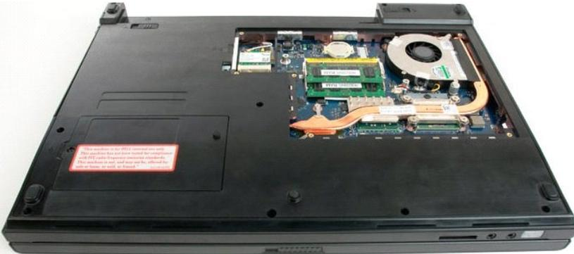
4. Insert scribe into slot and gently pry up the coin-cell battery.
