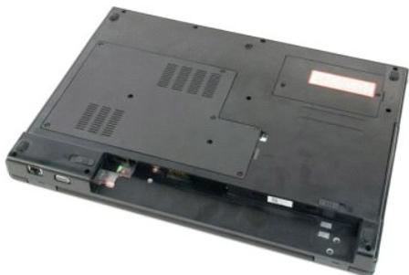
3. Remove the eight screws from the access panel.
