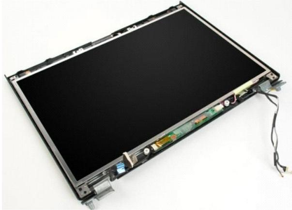
3. Disconnect the data cable from the display inverter.
