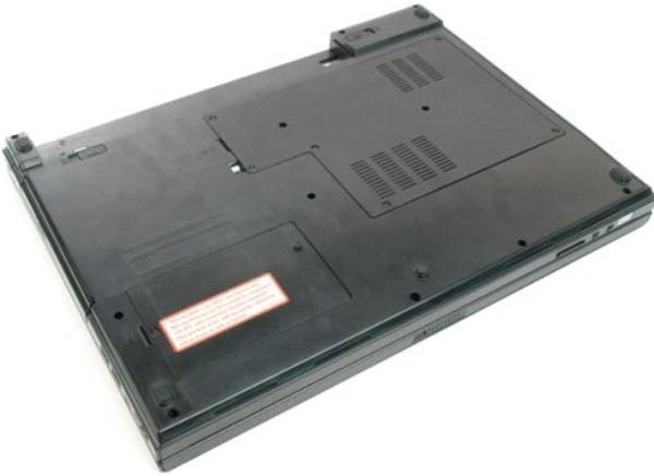
3. Remove the screw that secures the hard drive access panel to the base of the computer.
