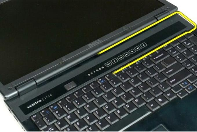
5. Continue to separate the hinge cover from the system working from right to left, then remove the hinge cover.
