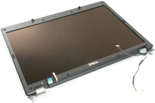
3. Remove the eight rubber screw covers from the display bezel.
