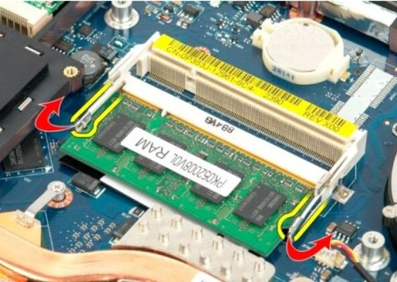
7. Slide the memory module out of the socket.
