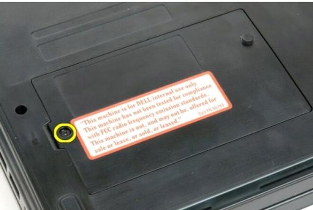
4. Insert a plastic scribe into the slot and lift up the access panel, then remove the panel from the computer.
