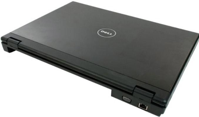
3. Use a plastic scribe gently to pry the back side of the hinge cover away from the base of the computer.
