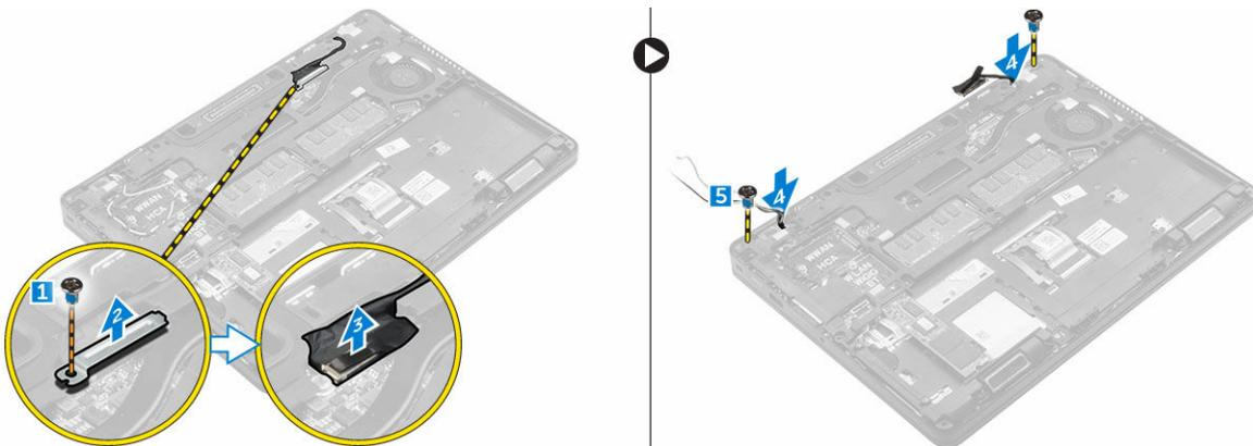
f Turn over the computer, open the display, and lift the display assembly from the computer [1] [2].
