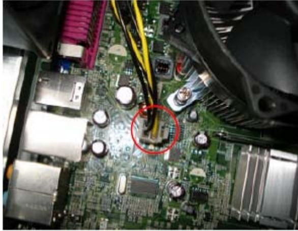
9. Disconnect P1 power cable and FDD data cable.
