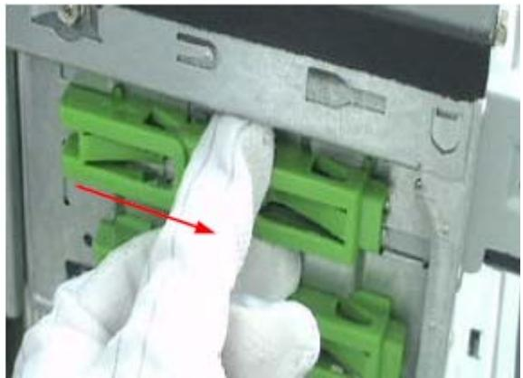
10. Install the FDD and slide the FDD rail to lock it.
