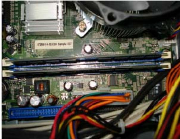
6. Fit the CPU cooler to the MB and fasten four screws shown.
