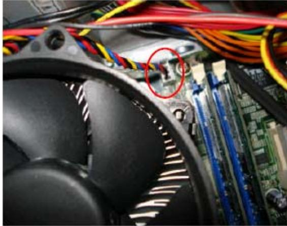
8. Connect the System Fan power-cable to the MB connector.
