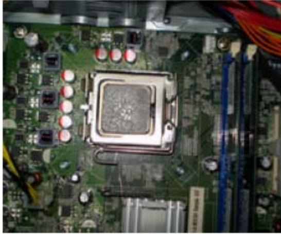
21. Remove the motherboard by releasing the six screws shown then lifting MB clear of the chassis.
