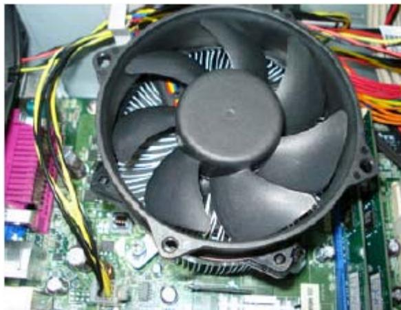
7. Connect the CPU Cooler power-cable to the MB connector.
