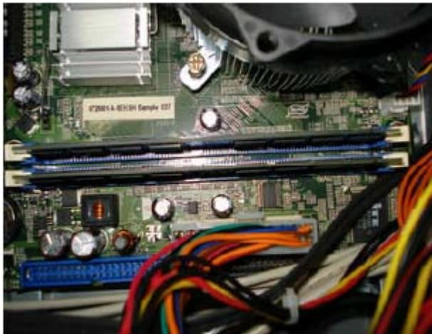
19. Remove the System FAN by releasing the four screws shown then removing the fan from the chassis.
