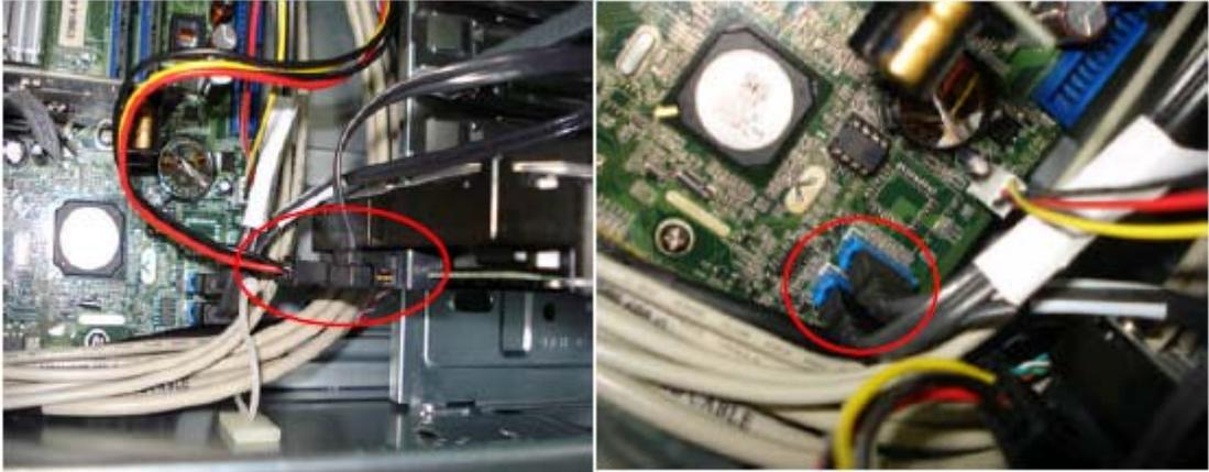
12. Disconnect the System Fan power-cable from the MB connector.
