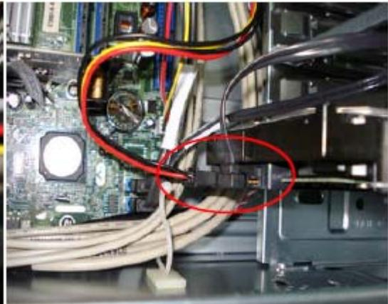
14. Connect the ODD data cable and power-cable to the rear of ODD.
